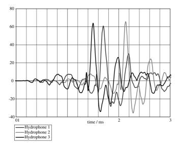
Fig. 2. A blast signal recorded by the hydrophone array showing the time delay caused by the shock wave reaching each hydrophone at different times. The shape of the signal recorded on each hydrophone is very similar for each event ensuring a sharp peak in the cross-correlation functions of pairs of signals.
