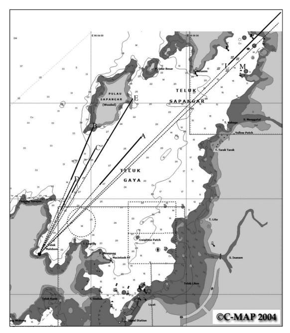
Fig. 1. The calculated bearing and range of seven of the blast events (A–E, L and M) recorded during this study. In each case, the thick lines represent the maximum and minimum distance to the blast's origin as estimated from the signal's peak pressure. Key: white—deep water, light grey—land, darker greys—shallow water. All depths in metres.
